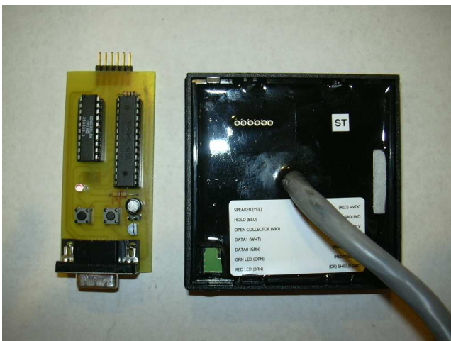
Figure 1. Register Capture Circuit shown with iClass RW300
